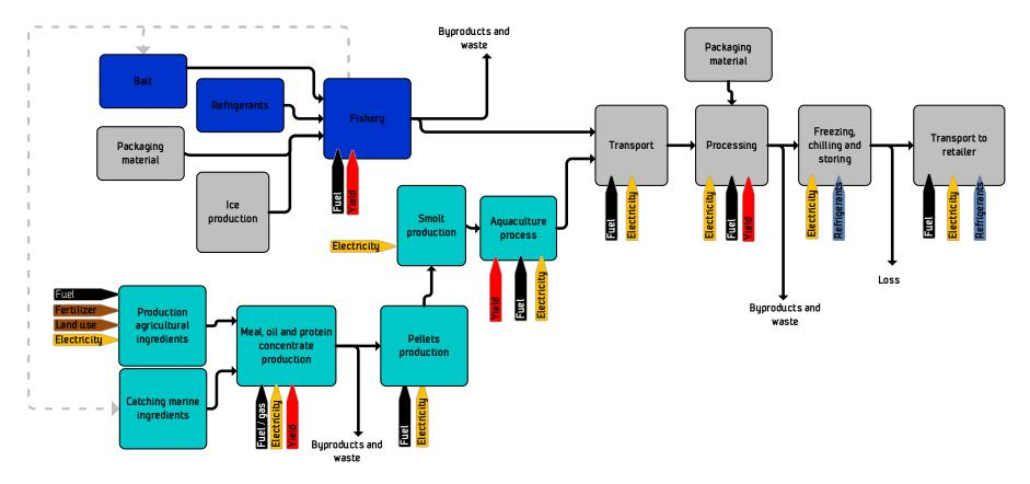
Figure 2-4 Example of flow chart for seafood production and distribution system from field and water to retailer gate. Direct emissions from the processes not included in this flow chart. The expected important mass and energy flows are indicated.
