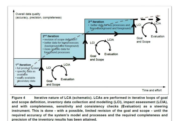
Figure 2-1 Illustration of the iterative LCA work flow from the ILCD handbook (EC-JRC, 2010)
