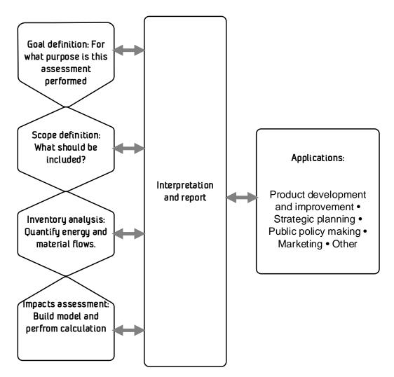
Figure 2-2 The phases of a GHG assessment/LCA
